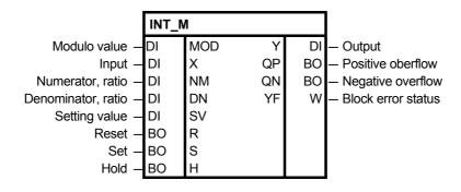
Brief description the virtual master block INT\_M is used to generate position reference
